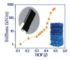
A macroscopic carbon nanotube (CNT) film with gradient structure is synthesized by one-step CVD. The CNT arrangement gradually changes from well aligned to random distribution in a continuous and smooth way along the thickness direction. Local deformation and mechanical properties such as stiffness and elastic modulus are determined by the Herman's orientation factor and span over three orders of magnitude.
