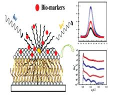
A novel method for ultrasensitive biomarker sensing is achieved by plasmonic bio-membrane templates for a wide range of fluorophores. Gold nanoparticle assemblies are used on lipid bilayer to get an emission enhancement through Förster resonance energy transfer. Furthermore, the role of nanoparticle membrane binding and penetration as well as its consequence on observed enhanced bio-fluorophore detection sensitivity is elucidated.
