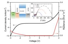
Light-emitting electrochemical (LECs) of organic-inorganic perovskite (CH3NH3Pbl3) with two high work function electrodes are demonstrated. Results indicate that CH3NH3PbI3 has an ionic conductivity of  $\approx 10^{-8}$  S cm<sup>-1</sup>. The accumulated ions at the interfaces result in a large capacitance, which suggests a potential application in electrochemical energy-storage devices, such as solid-state supercapacitors and batteries.
